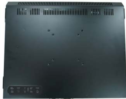
※Note 2:R07 (OSD Key on the back of the Monitor)
